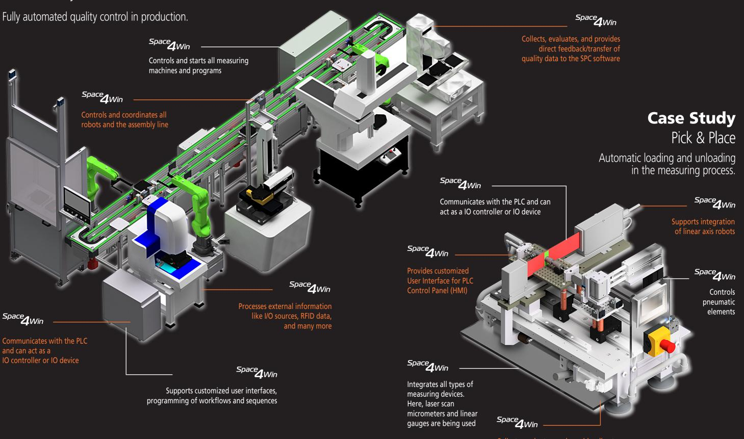
Collects, evaluates, and provides direct feedback/transfer of quality data to the SPC software
