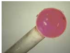
Contaminated stylus tip
