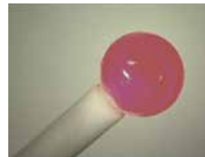
Cleaned stylus tip
